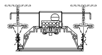
Square or rectangular CLIP-IN tiles are designed for installation in a grid of triangular profiles. Easy installation allows access to the space above the soffit for maintenance and inspection of installations.
