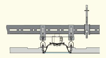
The suspended CLIP-IN ceiling system A/E uses a two-level supporting structure allowed to use of suspended ceiling panels of maximum dimensions  $2500 \times 600 \text{ mm}$  (1,5 m²) with the possibility of 100 % access to the interspace (including the folding variant).
