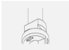
XTAK142-3, white Hook Base 2mm wire, white
